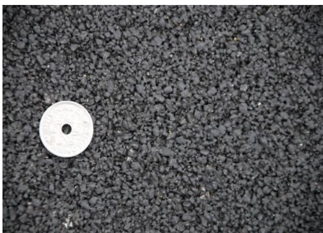
Rys. 9.12. Nawierzchnia jednowarstwowa (DVS-DRI Super Quiet Traffic International search for pavement providing 10 dB noise reduction, Danish Road Institute Report nr 178, 2009)
